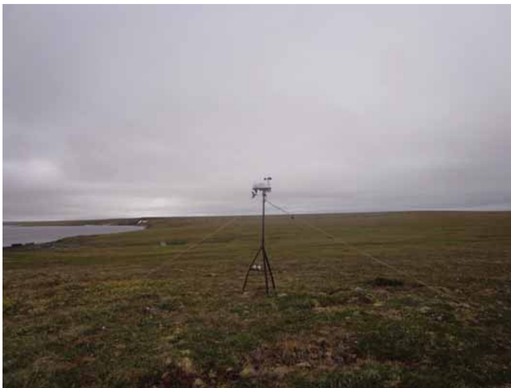
Figure 4.1-2: The Davis Vantage Vue meteorological station setup at Uomullyakh-Kyuel Lagoon camp on 2017-07-23
